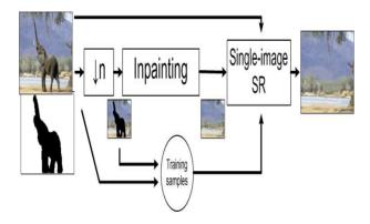
This system will be performing real time super resolution based inpainting. Initially the user will select the image on which he wants to perform editing. Then the region of interest is selected which user wants to edit. Then training samples are generated and dictionary is created. Once it is formed then the inpainting process begins and then eventually the desired image is formed.
